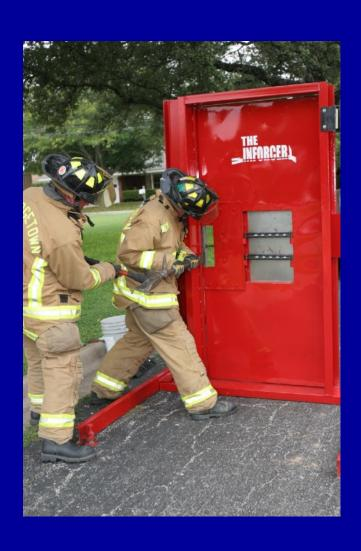
Works the tip of the tools around the edge of the Insert, always holding inward pressure
