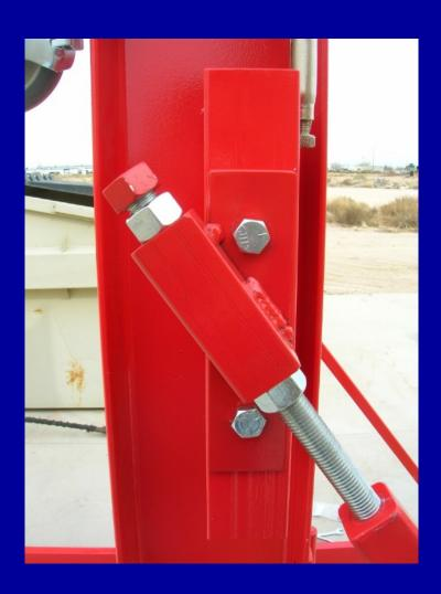
If needed nuts can be adjusted to adjust door
