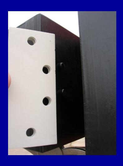
Place Hinge so hinge mounting holes align with Cut Station mounting pins
