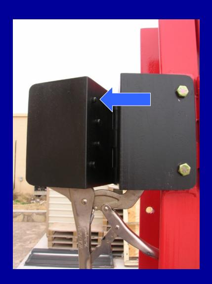
Open to expose Hinge mounting Pins
