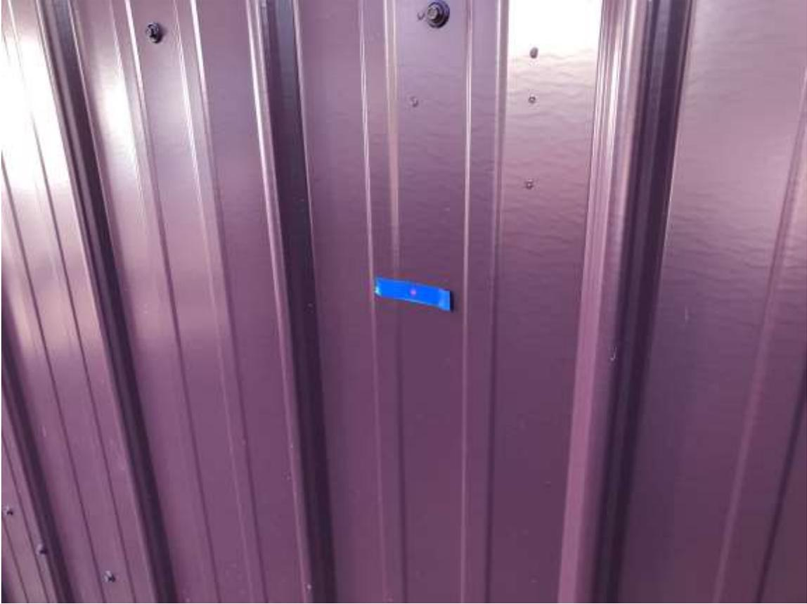
Above – Wall marking, in this case colored vinyl tape, placed where laser beam is identified on the structure and monitored for potential movement of the structure. The red dot showing on the blue tape is the laser beam from the tripod.
