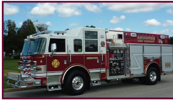
Squad 100 is a 2011 Pierce Arrow Rescue Pumper featuring a 1500 GPM pump with a foam system and a 10 KW generator.
